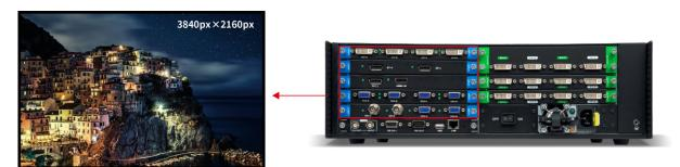
Each port  $4K \times 2K/60Hz$  or  $8K \times 1K/60Hz$
