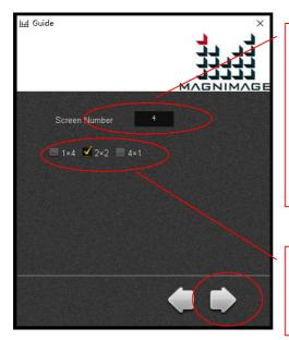
The number of parts to be spliced for the large screen. It means to put a few separate screens together, in this case the number of screens needs to be input, for example, a screen that needs 4 sending cards, and number 4 needs to be entered.
