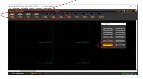
Use mouse to click one channel input source, then press the left key of the mouse to drag the source to the output. Thus we can achieve large spicing display requirements. Double click the layer, it can achieve quick full screen to this output port.
