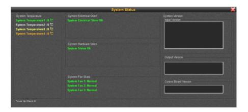
Upper machine software can monitor system, so users can check the system state real time. As above figure shows, the state includes: system temperature, electrical state, hardware state, fan state, firmware version, etc.
