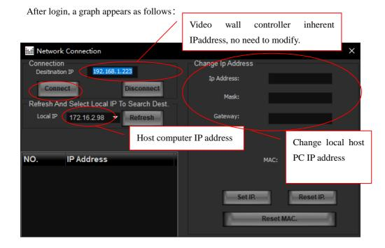
After the correct local IP address selected, please click "connect" button Hostcomputer software connection indicator in the bottom right of the interface.
