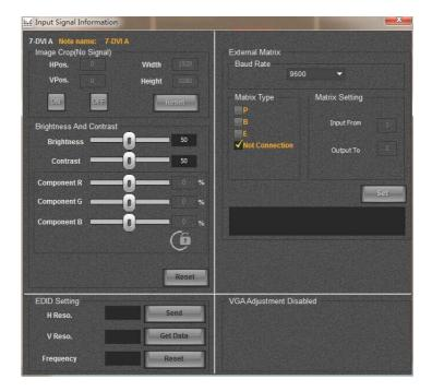
In this interface, we can adjust the parameters of the current input signal source, including image capture, brightness, contrast, EDID, VGA automatic correction, etc.
