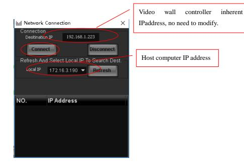
After the correct local IP address selected, please click "connect" button Hostcomputer software connection indicator in the bottom right of the interface.
