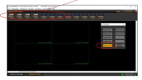
Use mouse to click one channel input source, then press the left key of the mouse to drag the source to the output. Thus we can achieve large spicing display requirements. Double click the layer, it can achieve quick full screen to this output port.
