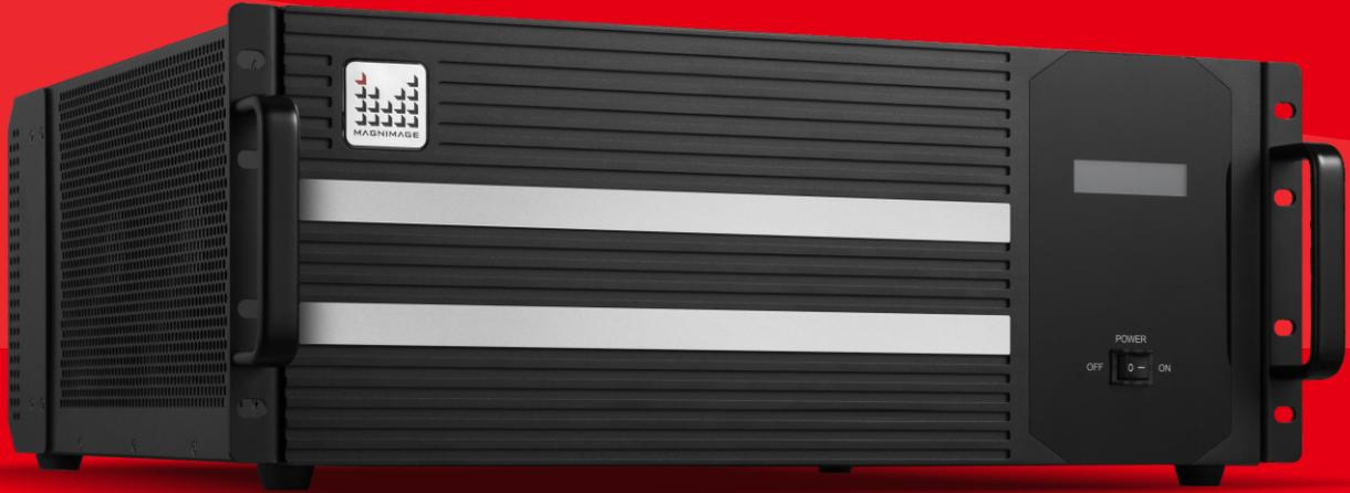
MIG-DN9404 is a video controller of full 4K input/output, the centerpiece of a large-screen splicing system. It can realize multiple input sources in different formats, and can be used for splicing, scaling, PIP, roaming, and overlaying on a variety of display terminals. The hardware architecture based on large-capacity, high-speed FPGA and a high-speed digital bus matrix ensures high signal reproduction and clear, smooth, latency-free output images.
